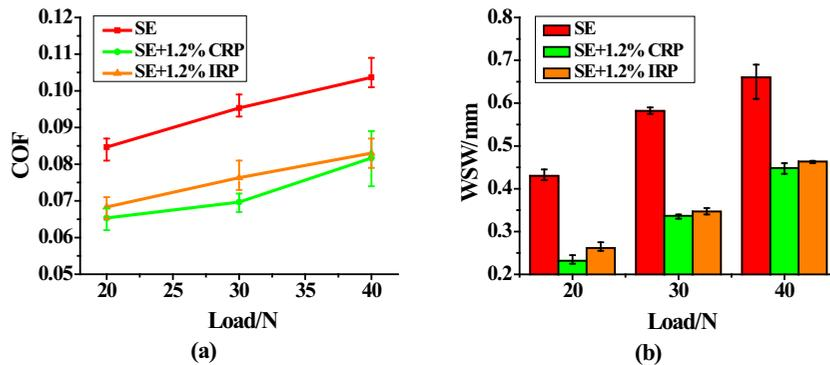
Figure 5 (a) COFs and (b) WSWs of the different mass fractions of CPN and IPN additives at 20 N
